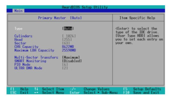
**NOTE:** Before attempting to configure a hard disk drive, make sure you have the configuration information supplied by the manufacturer of the drive. Incorrect settings may cause your system to not recognize the installed hard disk. To allow the BIOS to detect the drive type automatically, select [Auto].
